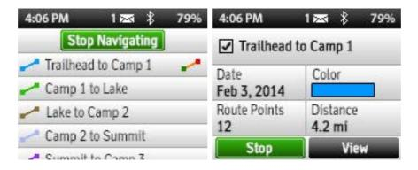
View the Details page for each route and turn routes on or off with a checkbox. Reverse routes by pressing the Reverse button on the Route Details page.
