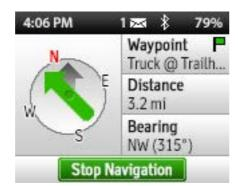
While Tracking: View your current speed, elevation, and heading with the Compass page along with a rotating compass graphic that shows your heading in relation to the cardinal compass points.
