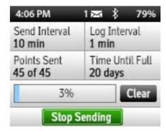
NOTE: Even when the Tracking Log is filled and begins overwriting older Track Points, a lower-detail tracking line is retained.
