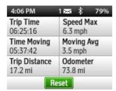
The accuracy of your Trip Info statistics depends on the frequency of your Tracking Log interval. A more frequent log interval will result in more readings and more accurate statistics.
