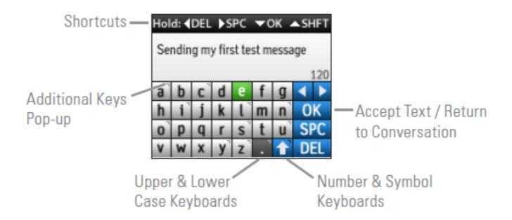
When using the keyboard hold the following buttons for special shortcuts:
