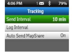
Adjusting the tracking intervals on inReach is not required, but doing so can offer greater flexibility depending on your trip speed and desired level of trip detail. inReach automatically records and stores tracking data in a trip log in the device's memory, whether or not you choose to send your track points to MapShare. Therefore, inReach allows you to adjust two different tracking intervals — a send interval and a log interval.
