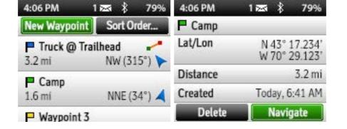
When navigating to a Waypoint, the Navigating icon appears next to the Waypoint label. It shows a green starting point, red finishing point, and orange connecting line.
