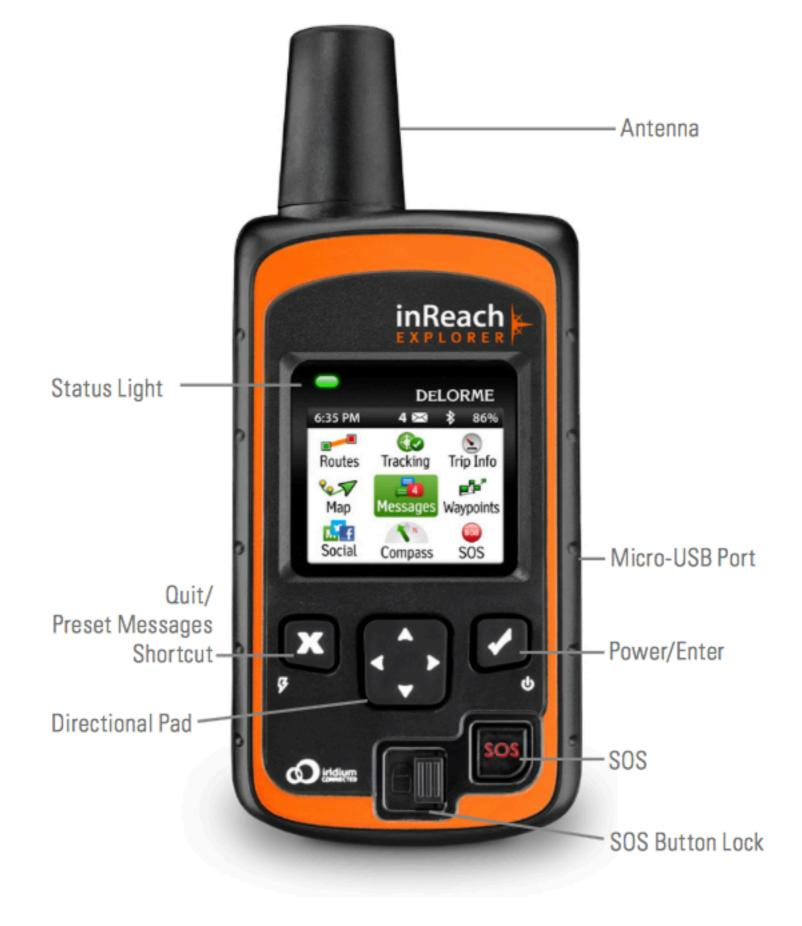
**Antenna** - When using the inReach Explorer, point the antenna up toward the sky and position the face of the device away from your body when attached to a pack or a vest.
